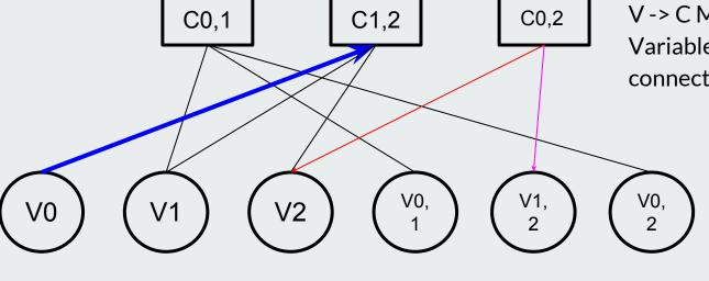
V -> C Message = probability of Variable's bit according the connected Check nodes
